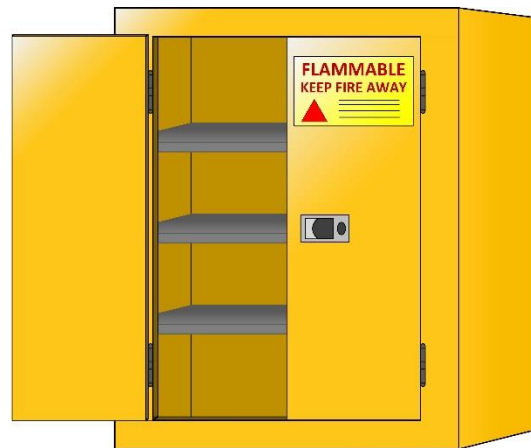
Figure 1 - Flammable Storage Cabinet
